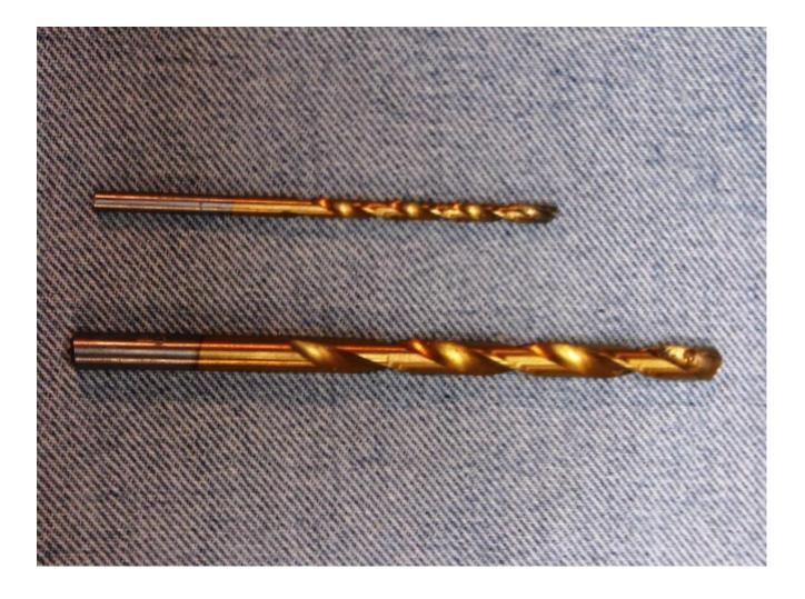
Use a HSS 1/8" drill for pilot drilling
