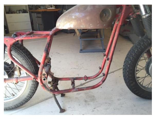
The center stand was junk and the side stand was missing... Incorrect brackets were removed and dents were removed - then off to the Blast Tech for sandblasting. It was put in a frame machine to verify correct alignment. Finally, it was off to Taint Paint for a coat of 80% gloss powdercoat.
