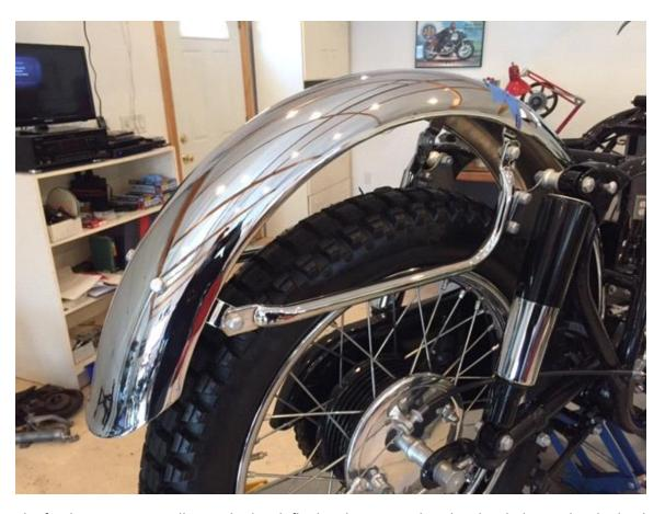
The fenders were originally attached with flat head screws rather than hex bolts, so they had to be made on the lathe and milling machine.
