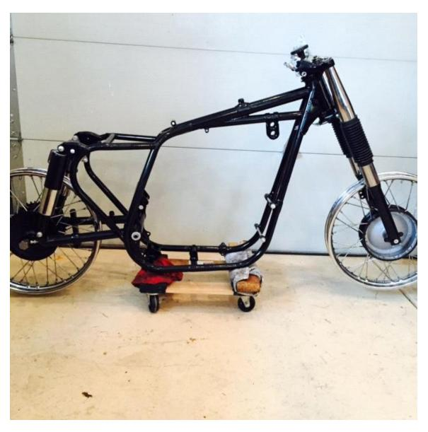
All new bushings and seals as well as new fork tubes were installed in the front suspension, and new rear shocks were sourced. I was able to find a genuine new old stock chain guard - what luck!
