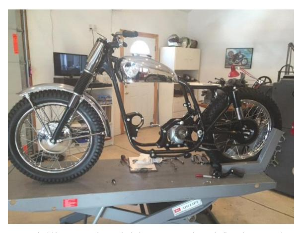
I starts to look like a motorcycle. I rebuilt the rare SC T2 gearbox with all new bearings. The engine was overhauled at the same time and it also received new bearings, pistons and valves. I was able to find a correct AMAL monoblock carburator so it was rebuilt and installed.
