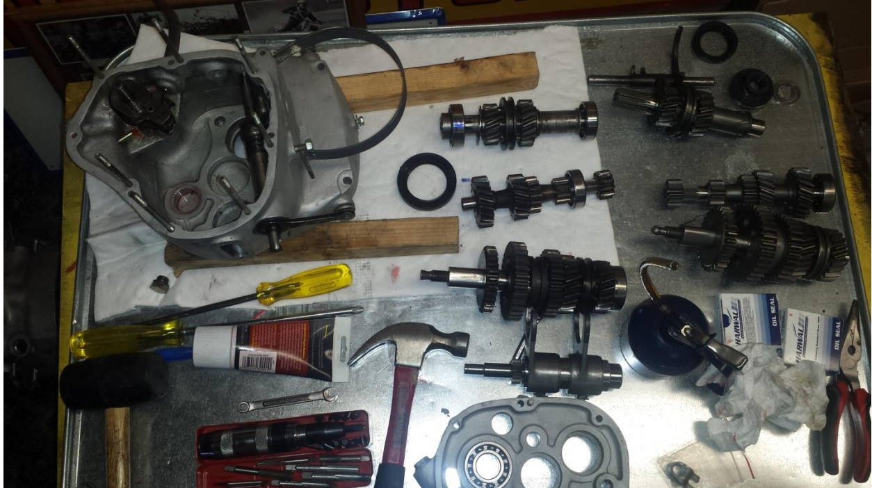
Transmission/transfer case ready for assembly
