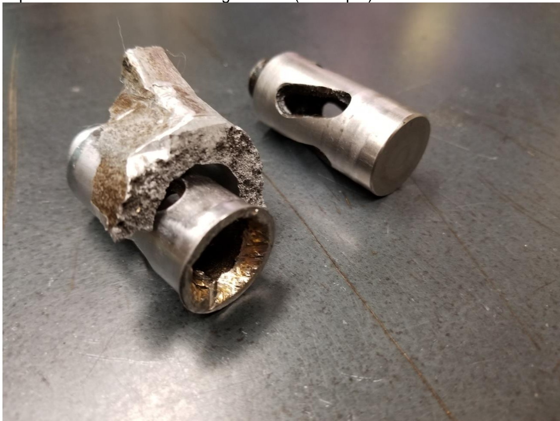
Wiped follower and chunk of engine case (the culprit)
